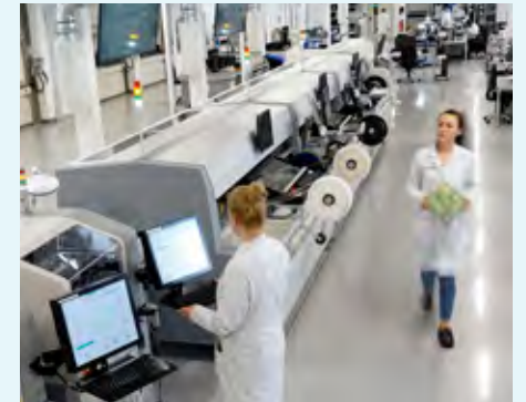
New full-line solution from Mycronic in action at Mikrolab, Germany, including two MY700 Jet Printers and three MY300 pick-and-place machines.
