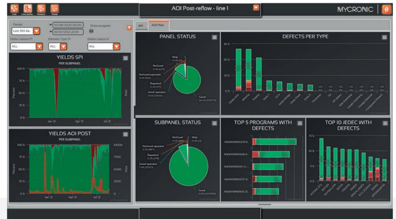
Print process quality has improved over the period but excessive warnings show we are operating close to process limits.
