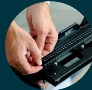
Handle short tape clips with the Tape Clip Magazine.
