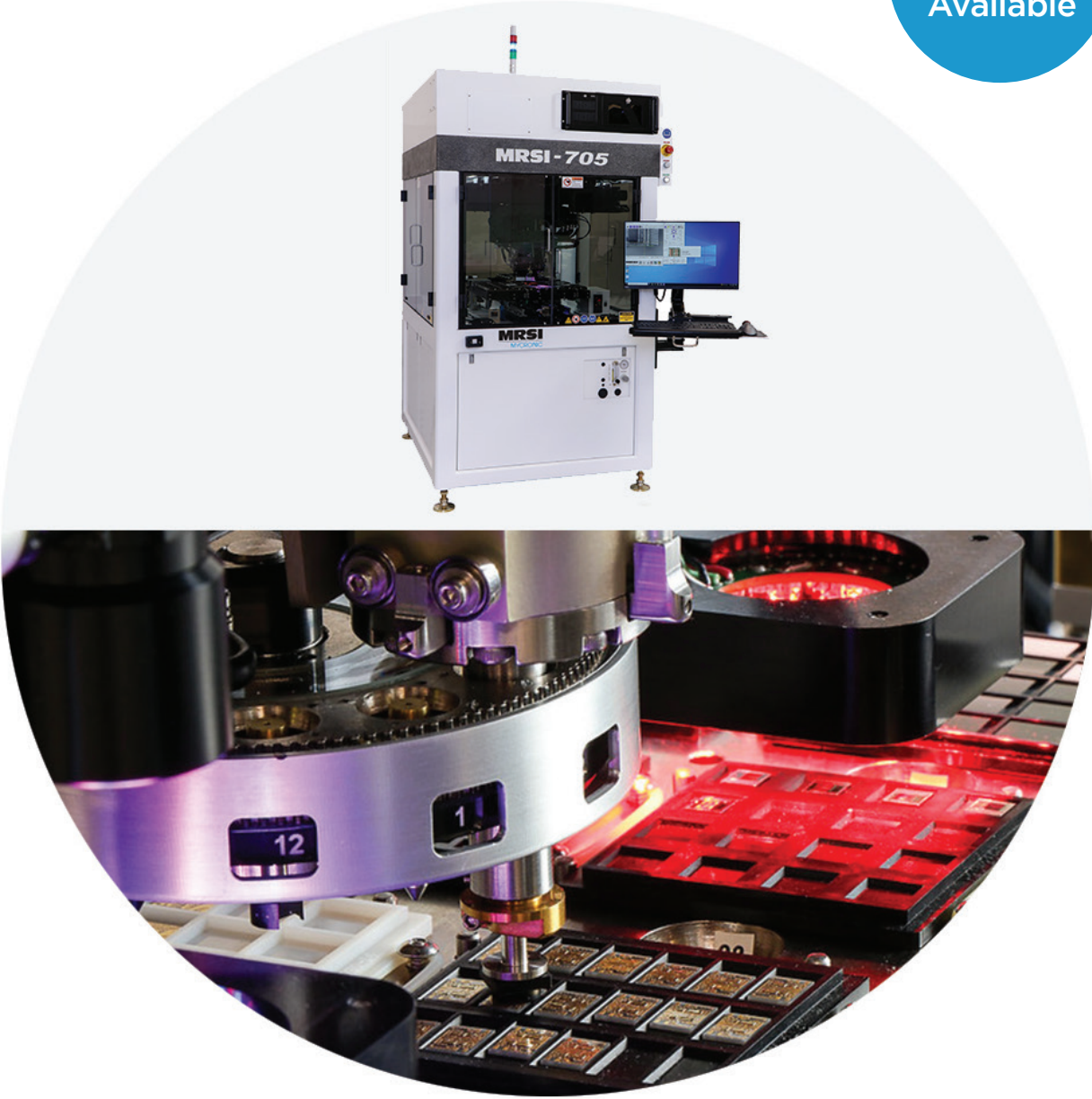
Patented turret for "on-the-fly" tool change
