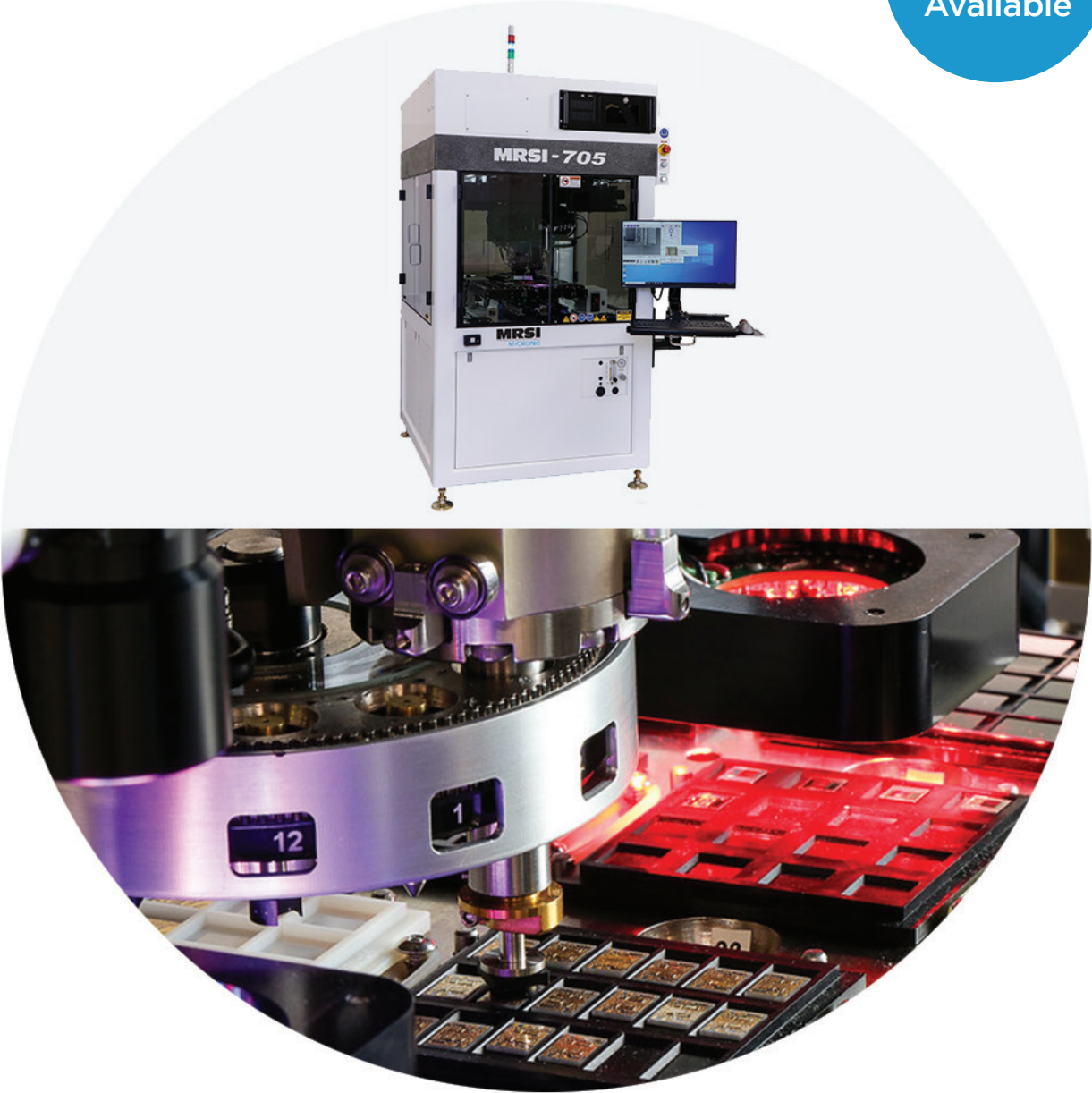
Patented turret for "on-the-fly" tool change
