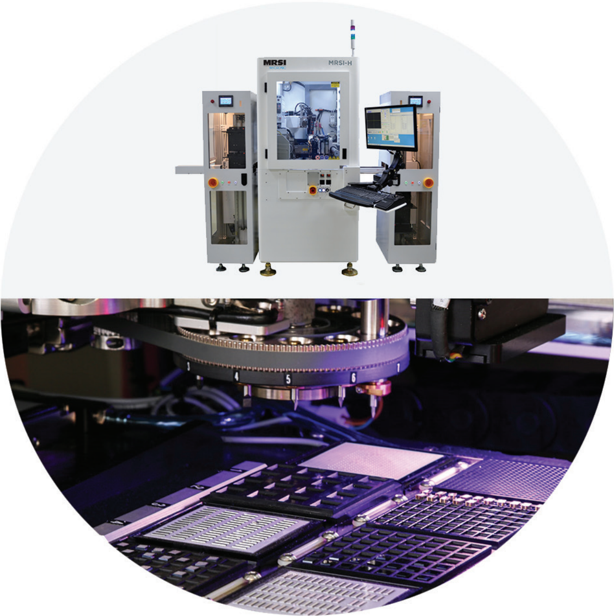
Patented turret for "on-the-fly" tool change
