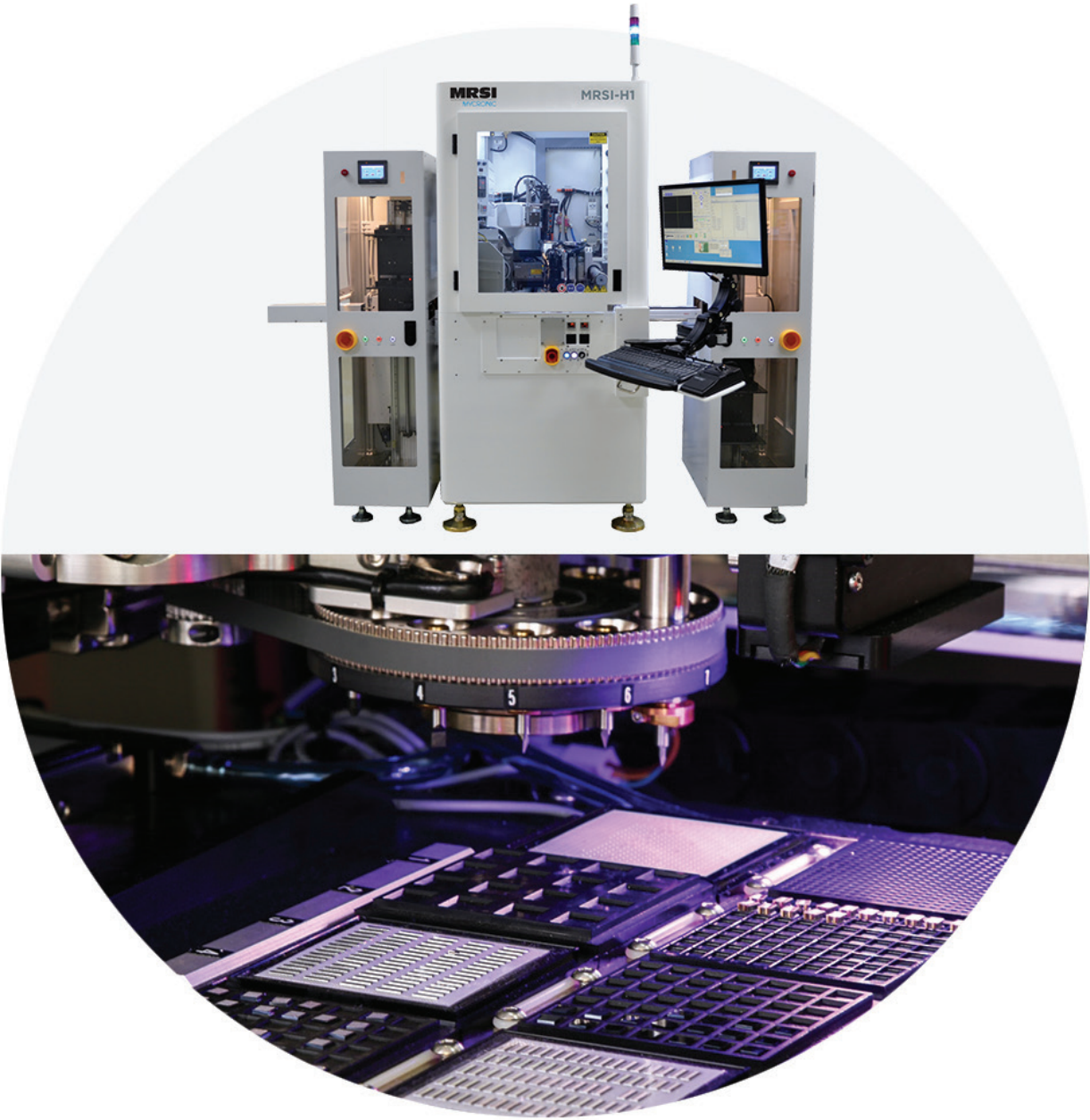
Patented turret for "on-the-fly" tool change
