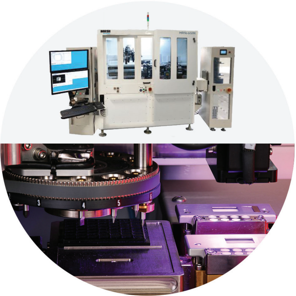
Patented turret for "on-the-fly" tool change
