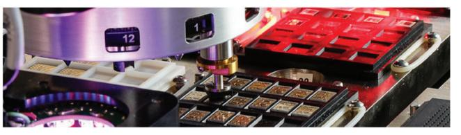
The MRSI-M3 offers an optional Turret configuration to significantly increase the speed and potential volume from our machine without sacraficing flexibility. This feature delivers an "on-the-fly" tool change with up to 12 tools with zero tool changeover downtime.
