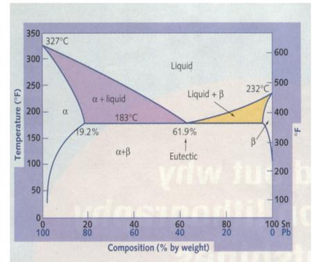
Figure 1: Eutectic transitions for a given metal composition—in this case, tin-lead.
