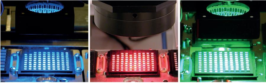
**Figure 5:** Programmable lighting intensity and color.
