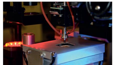
Figure 2: A pulse-heated, fast-ramp eutectic stage.
