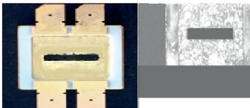
**Figure 4:** Eutectic package (left) with Sonoscan inspection results (right).
