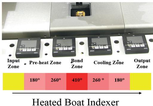
**Figure 3:** In-line eutectic die bonding.
