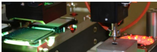
Figure 2: Eutectic bonding stage.
