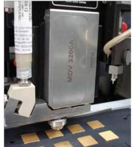
**Figure 2:** Jet valve on MRSI-175Ag dispense machine at the left, auger pump at the right.
